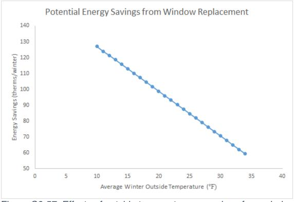
Figure C6-57. Effects of outside temperature on savings from window upgrade
