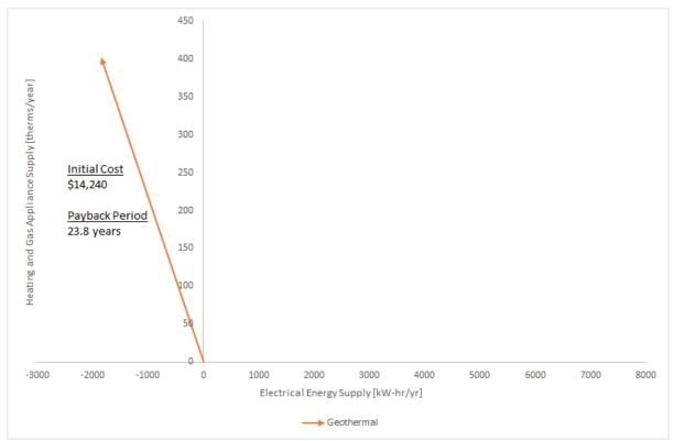
Figure A7.A8 Geothermal energy change
