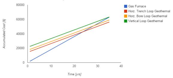
Figure A7.A13 Payback Period for Geothermal Alternatives
