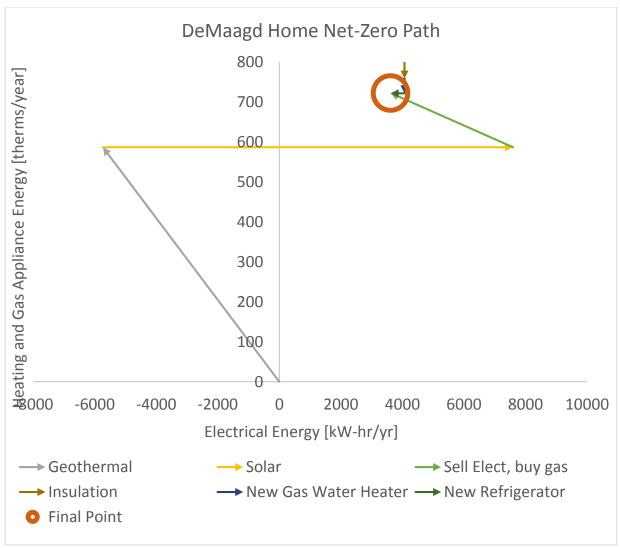
Figure 15: Combined energy saving/production path to net-zero home
