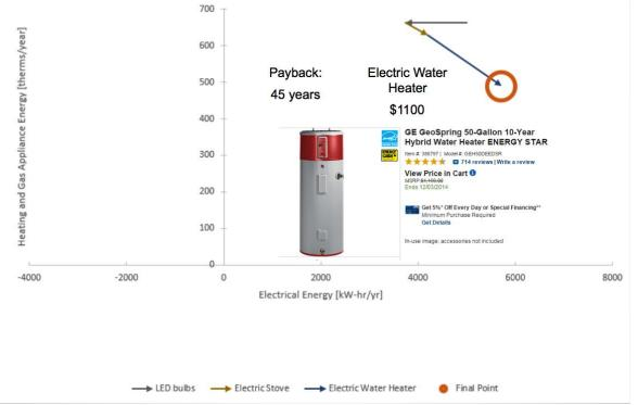
Figure A8: Effect of Electric Water Heater
