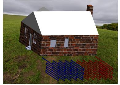
**Figure 9:** Geothermal field model mock-up. (Note: proposed geothermal field would be vertical, image is shown to illustrate location and general piping layout).
