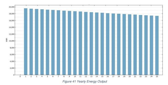
ag anargy output over the years is due to the degradation of solar t
