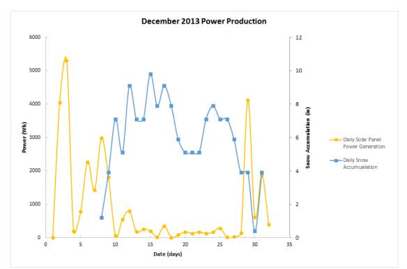
Figure C6-55. Comparison of solar panel energy generation and snow accumulation.
