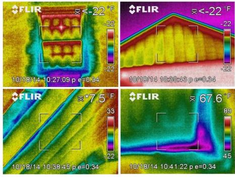
**Figure 5**: DeMaagd home IR camera pictures: outside rear window (top left), outside front wall (top right, inside west roof (bottom left), and inside basement exterior board (bottom right).
