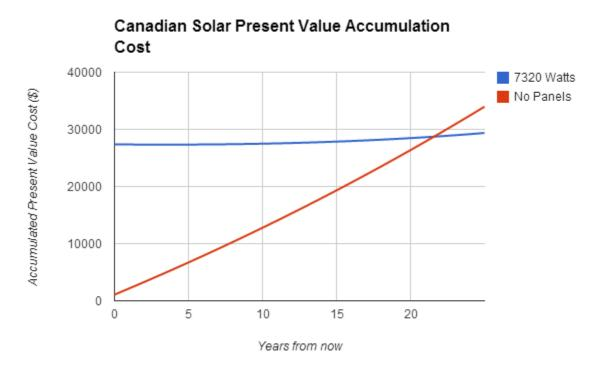
Figure A7.A9 Initial cost and payback period of a considered solar panel
