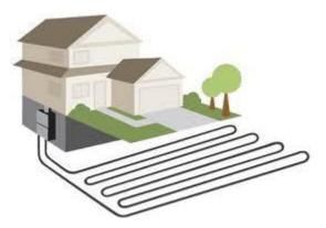
Figure 6 – Horizontal Geothermal Heat Pump
