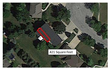
Figure A10: Area Required for Solar Panels
