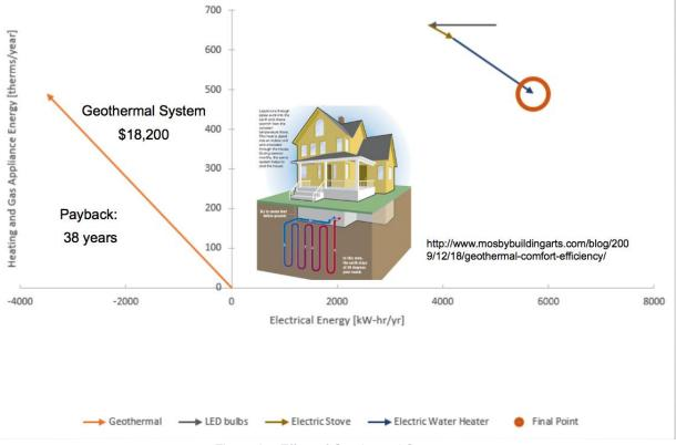
Figure A9: Effect of Geothermal System
