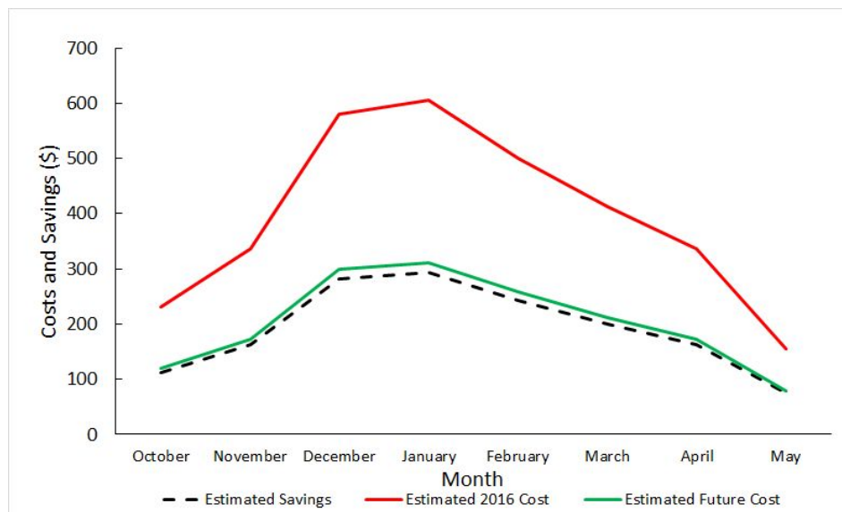
Figure C-6: Wall Insulation Costs and Savings
