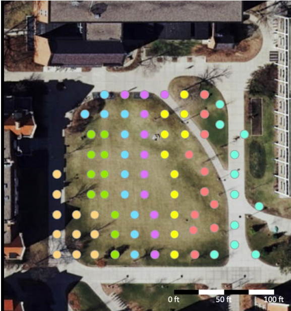
Figure E1: "Mini Bald Spot" Geothermal Field at Carleton College
